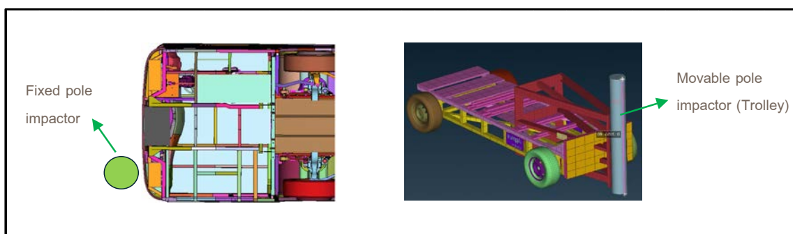
Figure 5.5: Illustration of test setting with a fixed pole impactor.
